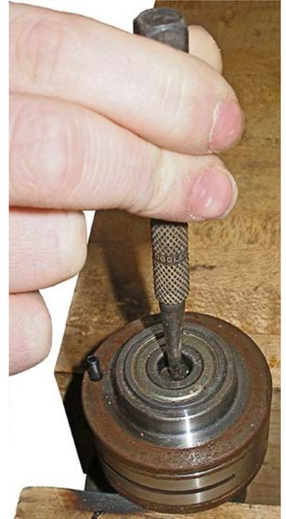
The eccentric bearing is pressed fairly tightly to the pad mount shaft. To support the bearing while I drove the shaft out, I placed 3 pieces of heavy sheetmetal in a triangle between the bearing and the flange of the pad mount, with the pad mount between the jaws of my bench vise. Then I drove the pad mount out of the bearing with a punch.
