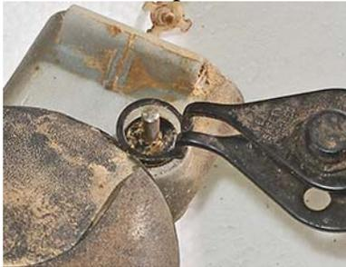
Remove the air lever by sliding the roll pin out of the housing. Unscrew the inlet bushing from the housing, and remove the spring, tip valve, and seal. Then, using a retaining ring spreader, remove the retaining ring from the top of the valve plunger, and slide the speed regulator out the bottom.
