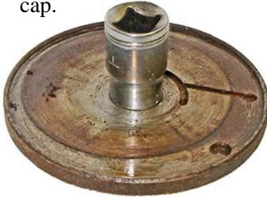
Turn the upper cylinder cap over, and drive the upper bearing out of the cap in a similar fashion. I found that a small socket would fit through the cylinder cap, but not the bearing, so this worked well for driving the bearing out of the cap.
