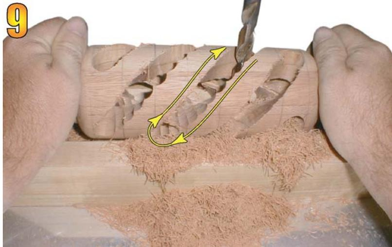
Smooth the rough-cut spirals. If you don't have a sanding drum small enough to fit the spiral, you can use the side of a drill bit. Make sure you work in a clockwise direction for better control.
