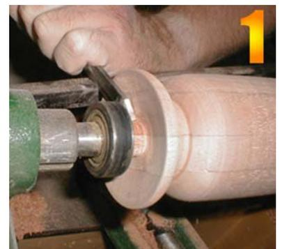
**Dish Out the top flange with a parting tool to create a cradle for the candle.**
