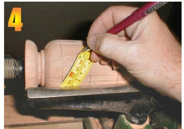
Use a flexible straightedge to draw the spiral layout lines.
