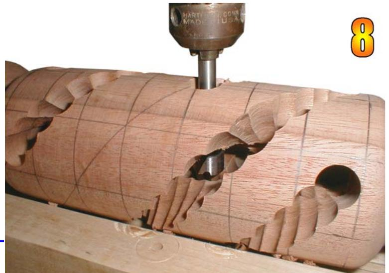
These candle holders also have a couple of big brothers. To make these 4" by 4" spirals, I mounted the drillpress on a carriage that rolls across the lathe bed.
